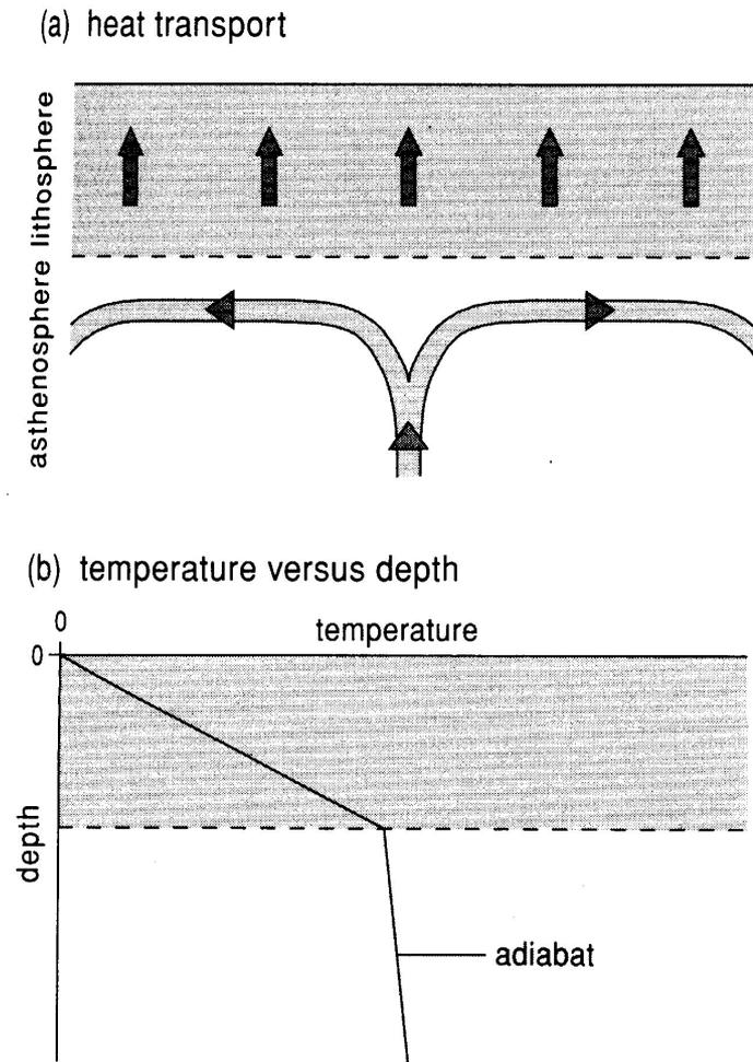
**Figure 17.2** Heat transport within the Earth (schematic).
