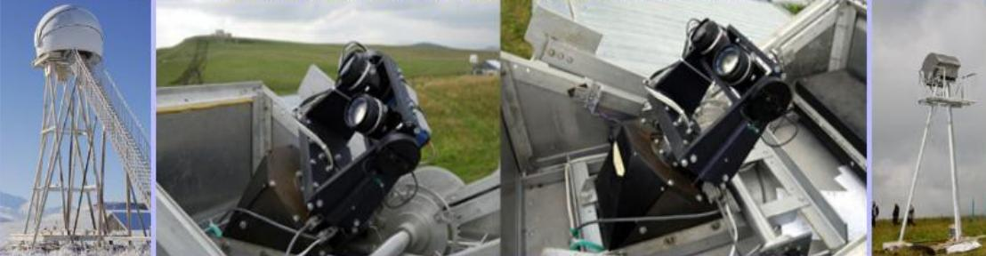
*MASTER II (8 square degrees) + MASTER VWF-4 Very Wide Field Cameras (FOV (max) = 4 x 25.5 x 39.8 = 4060 square degrees, Time resolution up to 150 ms, 4 CCD 11 Mpix*
