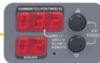
At-the-rack power monitoring of current (amps), voltage and active power (watts)
