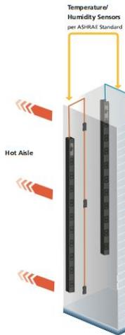
Specifically, eBay provides 400V 3-phase Raritan intelligent rack power distributed as "plug strips" or "rack PDUs" in each PDU, with internal line-to-neutral (3-pin) supplies each server with 240V, single phase within the operating range of the power any IT equipment.
