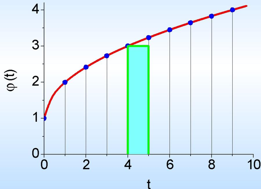
$$\Delta c_i(x, t) = \varphi(t_i) \left[ \operatorname{erfc} \frac{x}{\sqrt{4D(t-t_i)}} - \operatorname{erfc} \frac{x}{\sqrt{4D(t-t_i-\Delta t)}} \right]$$
