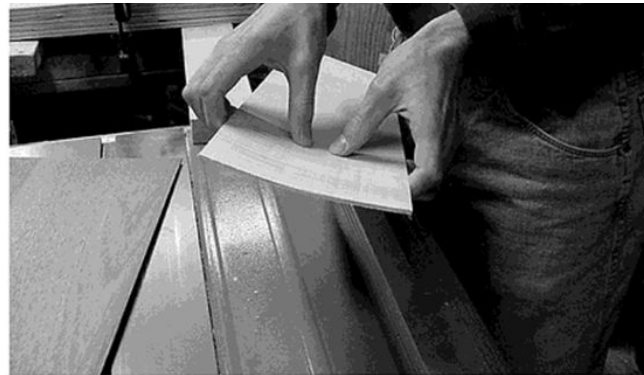
Figure 7.14 Checking a Piece of Wood by Flexing Across the Grain
