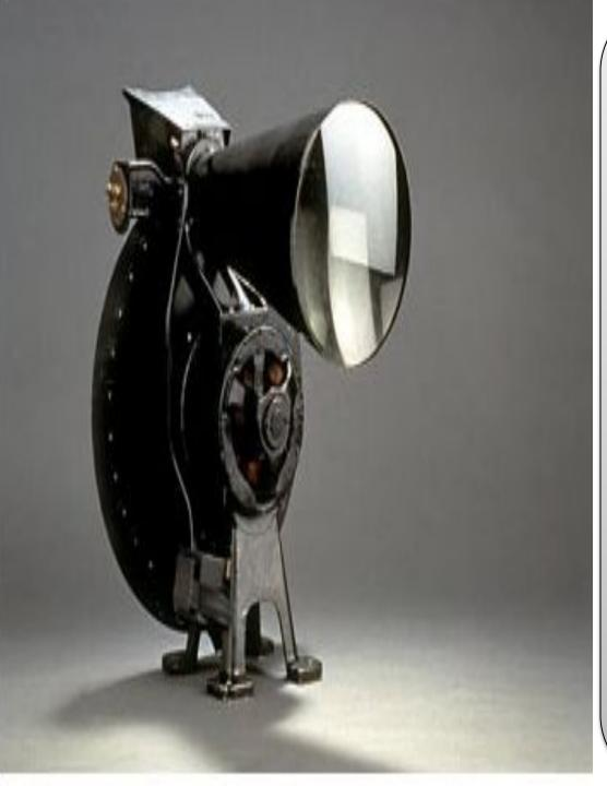
In 1884 Paul G. Nipkow, a 20-year old university student in Germany invented the first electromechanical television system which employed a scanning disk, a spinning disk with a series of holes spiraling toward the center, for rasterization.
