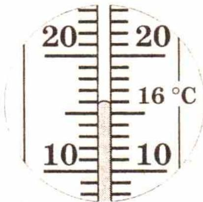
$$\text{цена деления} = \frac{20\text{ }^{\circ}\text{C} - 10\text{ }^{\circ}\text{C}}{10} = 1\text{ }^{\circ}\text{C}$$
