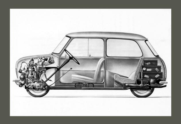
To do this, it used a transverse arrangement of a water-cooled four-cylinder engine, under which a gearbox was placed combined with an oil sump. The machine was equipped with front-wheel drive, which helped to reduce the weight. In addition, the model received 10-inch wheels.
