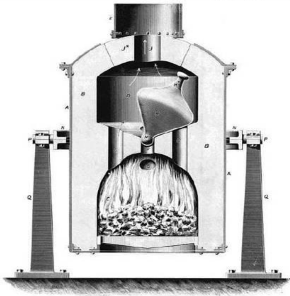
FIG. 24. BESSEMER'S FURNACE FOR THE MANUFACTURE OF OPTICAL GLASS
