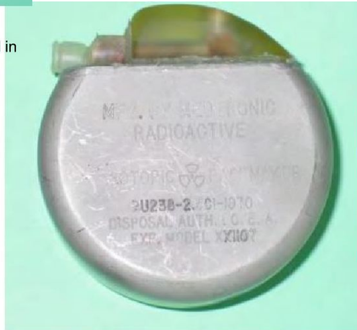
Figure 3 - This Medtronic nuclear pacemaker still “ticks” 35 years after it was manufactured.
