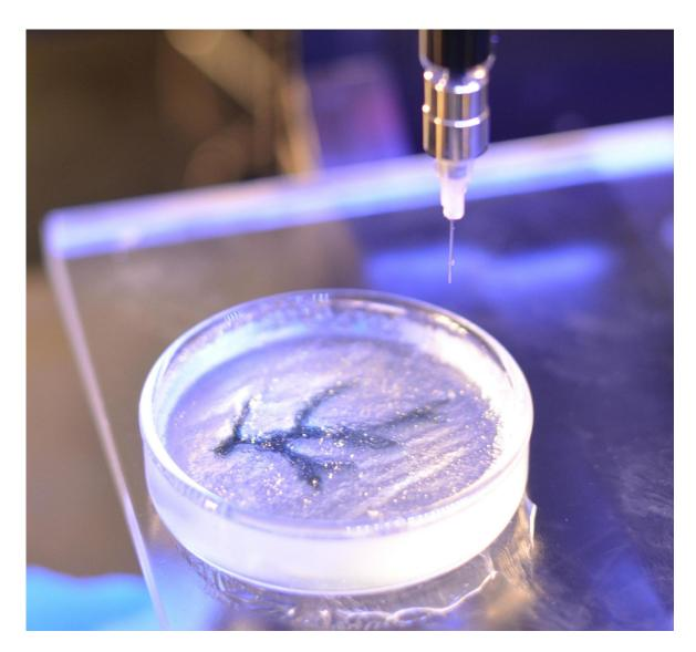
•One of the many types of 3D printing that is used in the medical device field is bioprinting. Rather than printing using plastic or metal, bioprinters use computer-guided pipette to layer living cells, referred to as bio-ink, on top of one another to create artificial living tissue in a laboratory.
