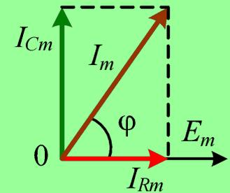
$$\left\{ \begin{array}{l} I_m^2 = (E_m/R)^2 + (\omega CE_m)^2 \\ I_m^2 = I_{Rm}^2 + I_{Cm}^2 \end{array} \right.$$
