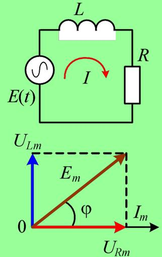
$$E(t) + E_{Si} = U_R \quad E(t) = IR + L \frac{dI}{dt} \quad \left\{ \begin{array}{l} I(t) = I_m \cos \omega t \\ E_{Si} = -L \frac{dI}{dt} \end{array} \right.$$
