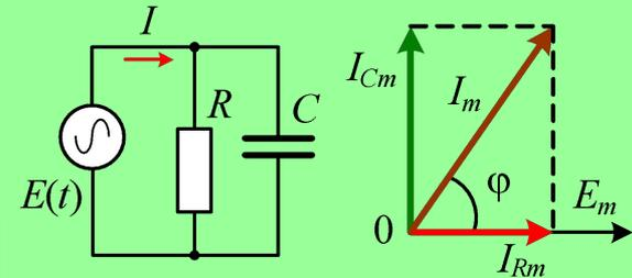
$$I_m^2 = (E_m/R)^2 + (\omega C E_m)^2 \quad Z = \frac{E_m}{I_m} = \frac{R}{\sqrt{1 + (\omega C R)^2}}$$
