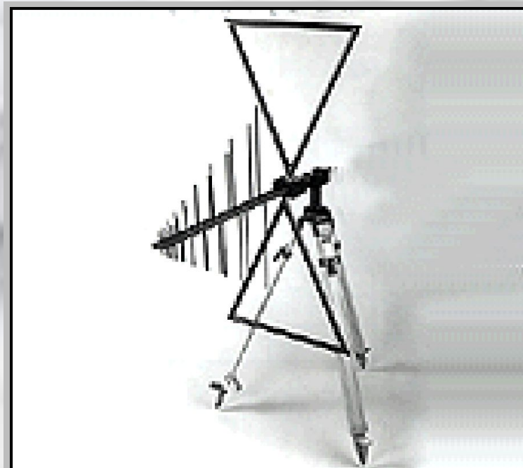
HP 11966P broadband antenna, 30 MHz to 1 GHz
