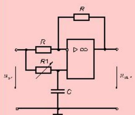
$$\varphi = -2 \arctg(\omega R_1 C)$$
