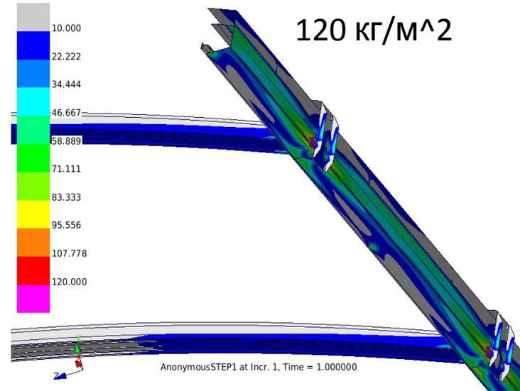
Element: Stress components (S): Von Mises @ SNEG
