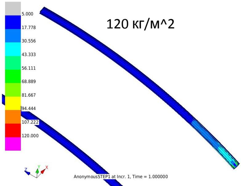
Element: Stress components (S): Von Mises @ SNEG
