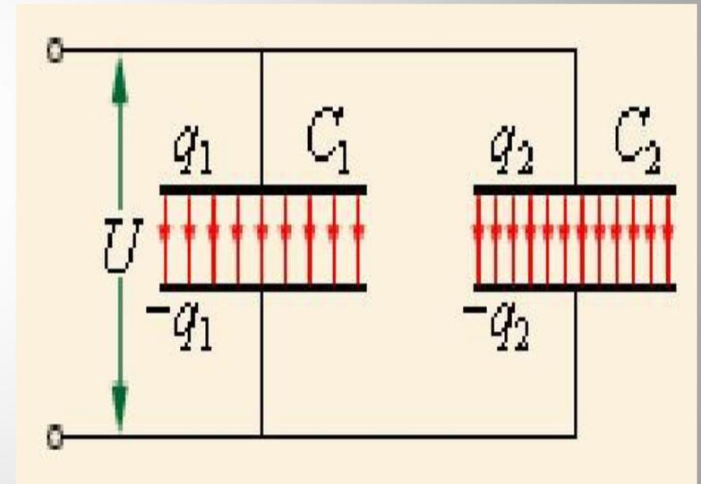
$$C = \frac{q_1 + q_2}{U} \quad \text{или} \quad C = C_1 + C_2$$
