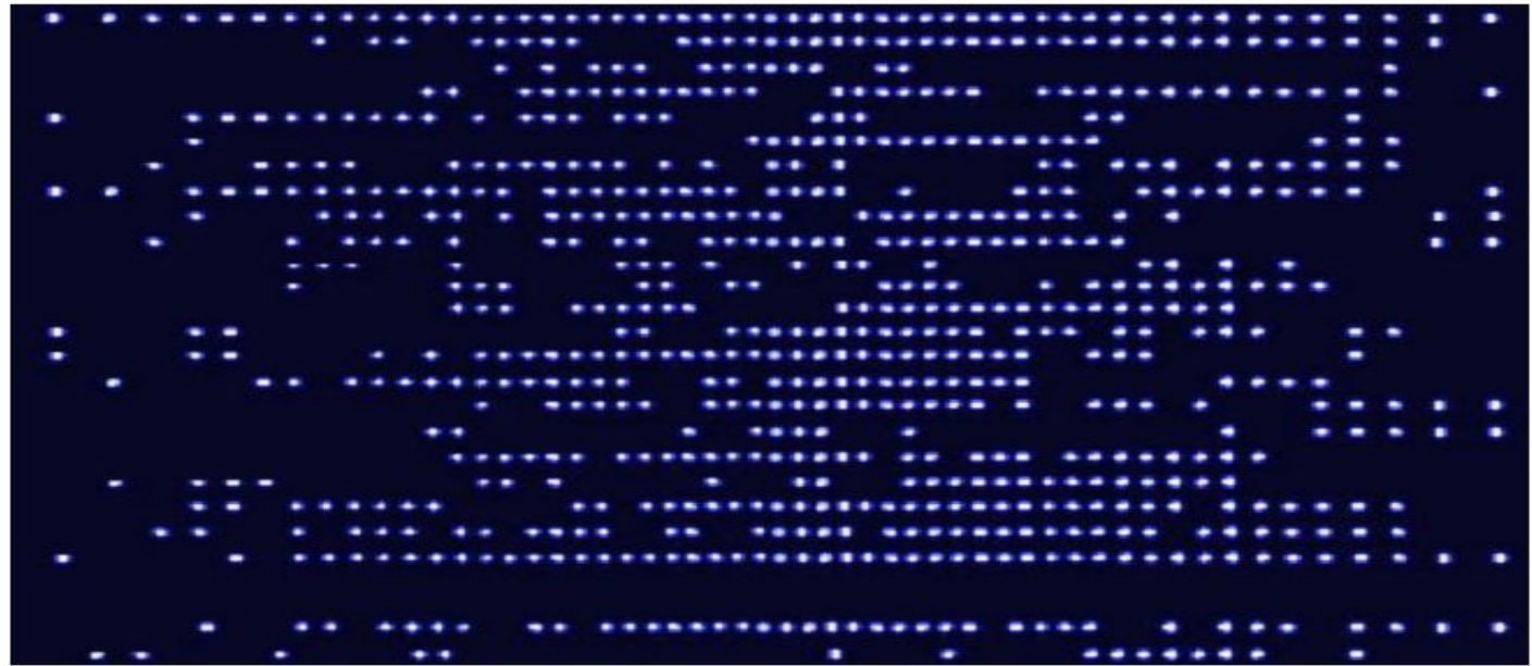
Complex qubit organization: each row is a separate image of 53 trapped ion qubits, with each qubit fluorescing (state 1) or dark (state 0) upon measurement.,
