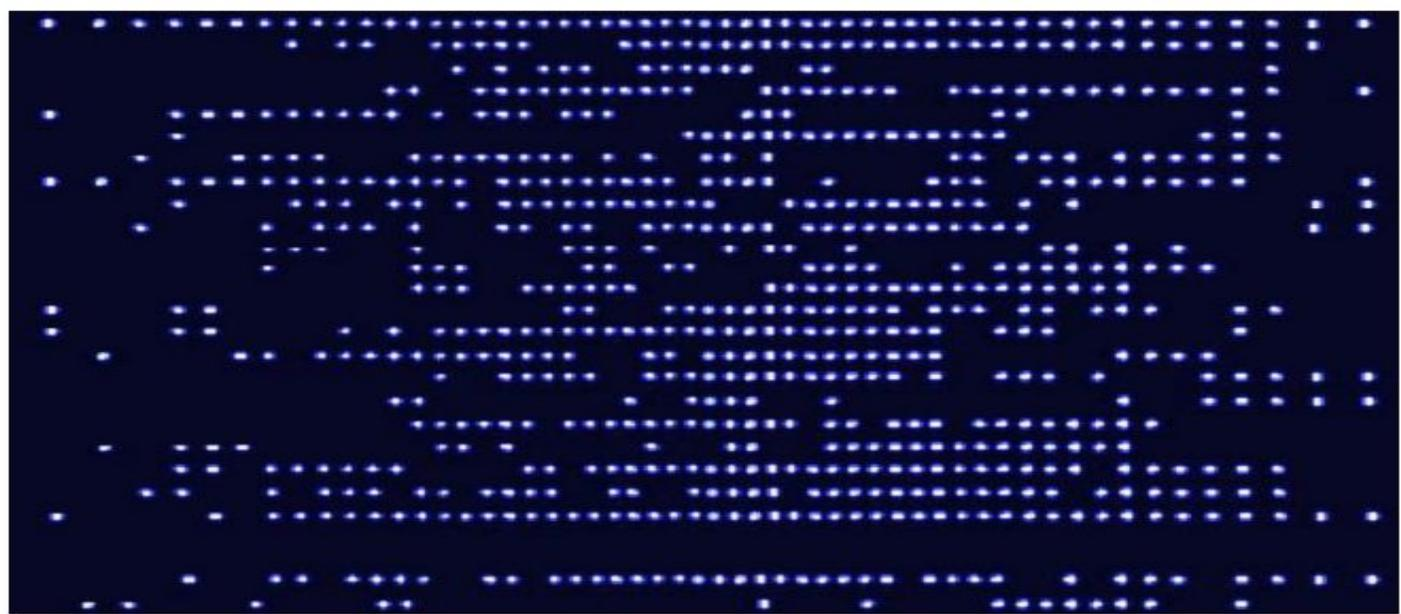
Complex qubit organization: each row is a separate image of 53 trapped ion qubits, with each qubit fluorescing (state 1) or dark (state 0) upon measurement.,
