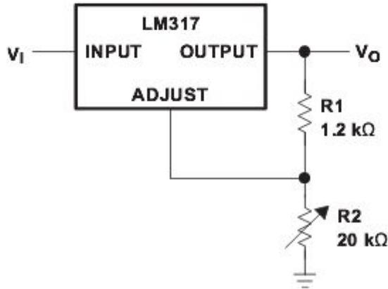
$$V_O = V_{REF} (1 + R_2/R_1) + I_{ADJ} R_2$$
