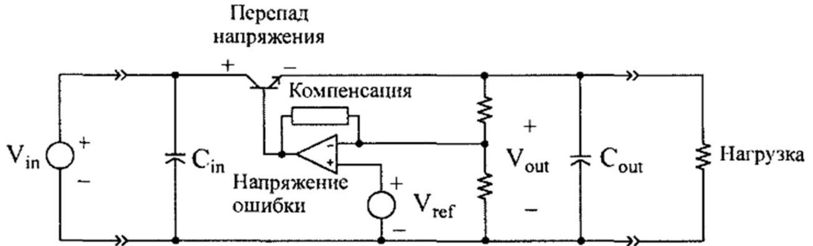
$$P_{HR} = (V_{in(max)} - V_{out}) * I_{load(rated)}$$
