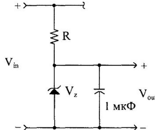
$$V_{in(min)} > V_{out} + 3V$$
