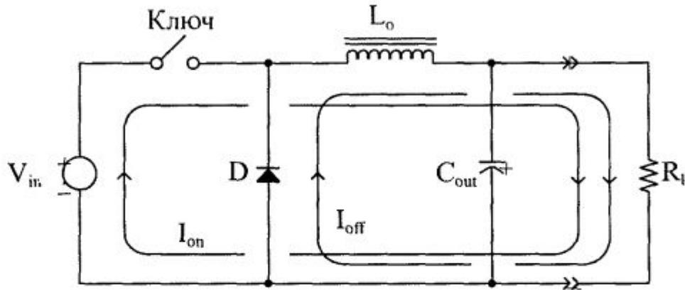
$$V_{out} = V_{in} * T_{on} / T_{all}$$
