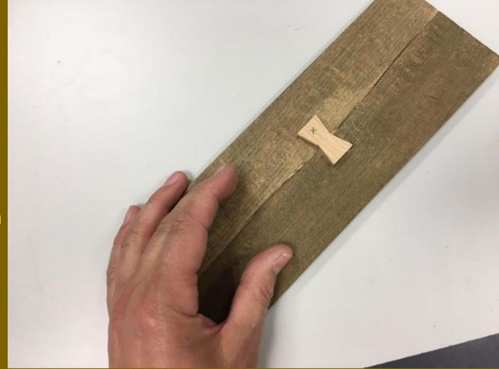
First make a dovetail of wood, ca 4-5mm thick.
