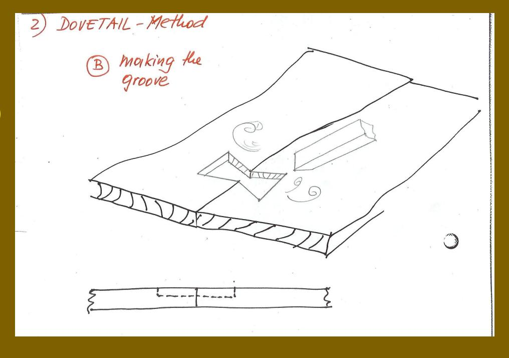
Glue the groove, then place in the dovetail-piece.
