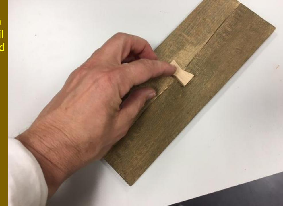
For additional strengthening a wooden dovetail can be made and glued into a groove on the boards
