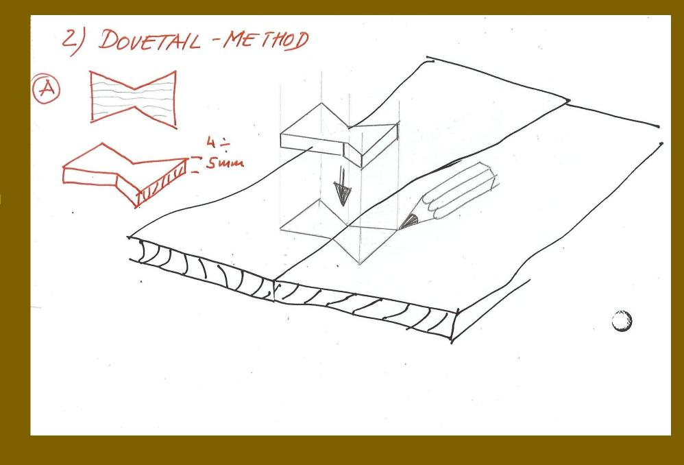
Now make the groove, by use of a sharp crowbar (лом)
