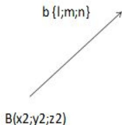
$$d = \frac{\sqrt{\left| \begin{matrix} x_2 - x_1 & y_2 - y_1 \\ l & m \end{matrix} \right|^2 + \left| \begin{matrix} y_2 - y_1 & z_2 - z_1 \\ m & n \end{matrix} \right|^2 + \left| \begin{matrix} x_2 - x_1 & z_2 - z_1 \\ l & n \end{matrix} \right|^2}}{\sqrt{l^2 + m^2 + n^2}}$$
