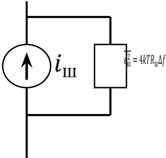
$$\overline{e_{\text{ш}}^2} = 4kTR_{\text{ш}}\Delta f$$
