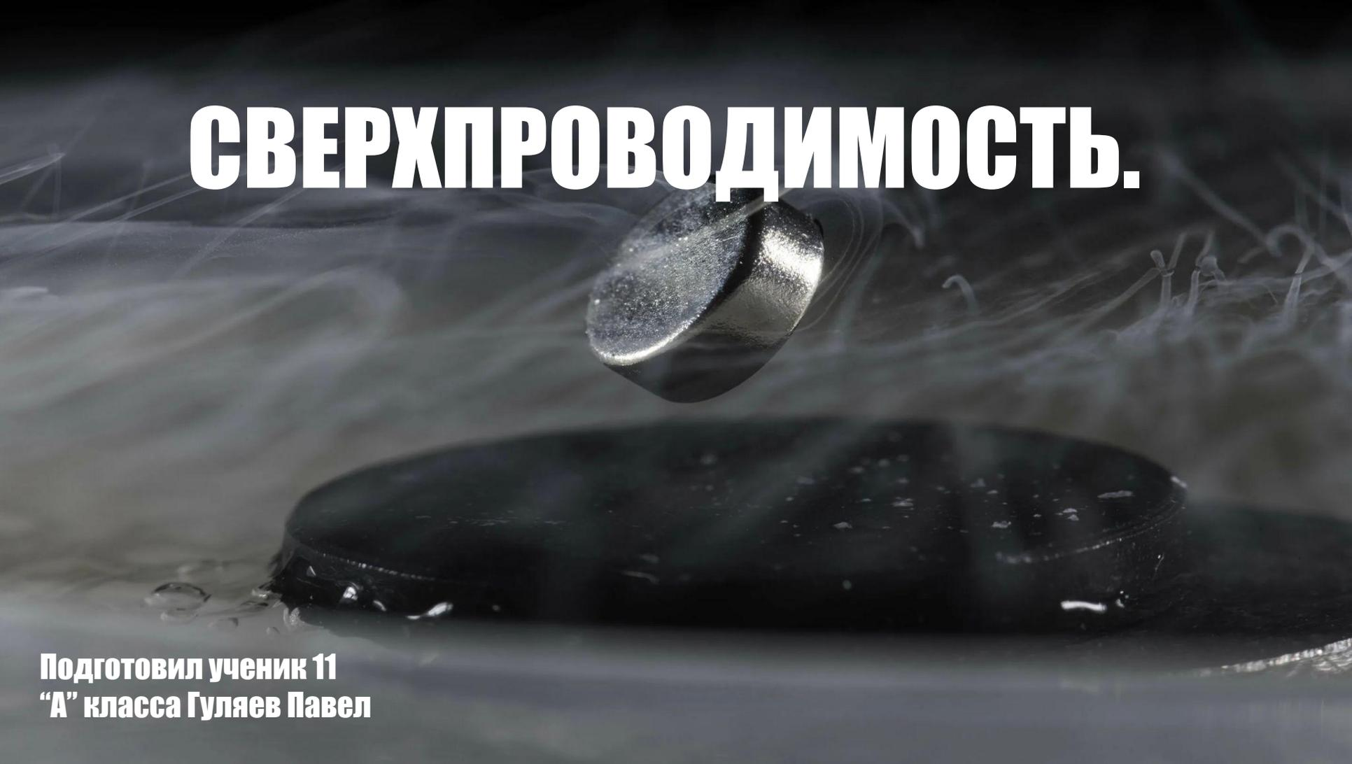
A black and white photograph showing a small, cylindrical, metallic superconductor levitating above a larger, dark, circular superconductor. The levitation is achieved through the Meissner effect, where the superconductor repels the magnetic field of the magnet below it. The background is dark and slightly hazy, emphasizing the levitating object.
