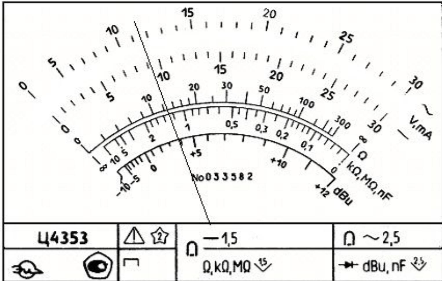
$V_- = 120 \text{ B}; mA_- = 3; \Omega; k\Omega \times 1; k\Omega \times 100;$
