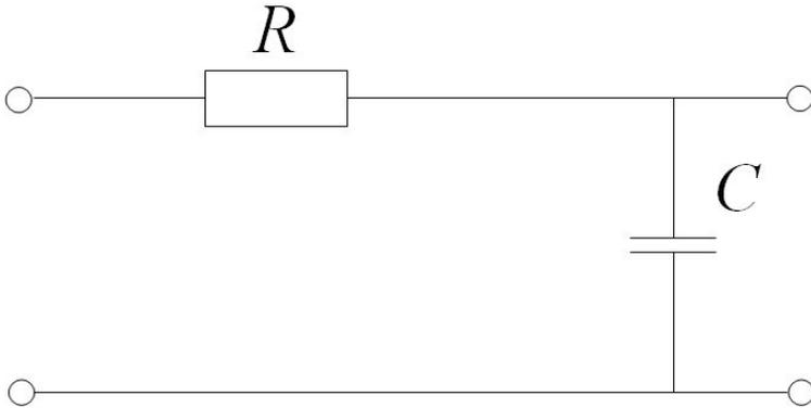
$$x(t) = i(t)R + y(t), \quad i(t) = C \frac{dy(t)}{dt} \Rightarrow$$
