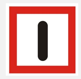
• **Damming plant** It can be approached at a distance marked on the board. (e.g. 300 m)
