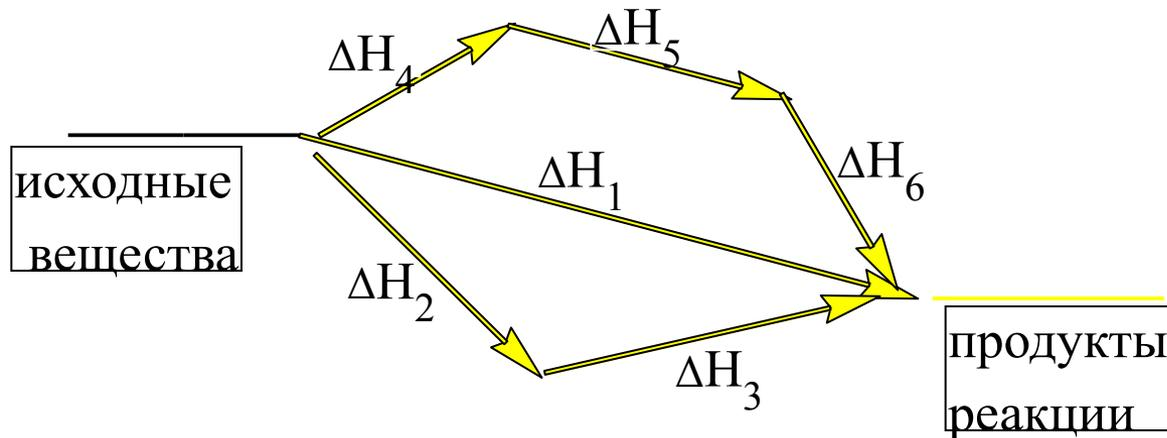
$$\Delta H_1 = \Delta H_2 + \Delta H_3 = \Delta H_4 + \Delta H_5 + \Delta H_6$$
