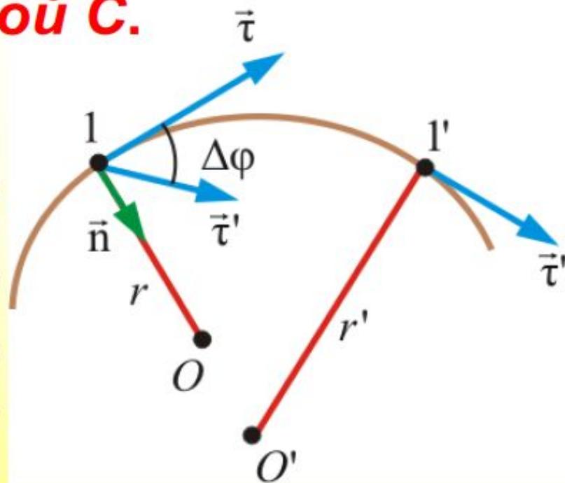
$$r = \frac{1}{C} = \lim_{\Delta\varphi \rightarrow 0} \frac{\Delta S}{\Delta\varphi} = \frac{dS}{d\varphi}.$$
