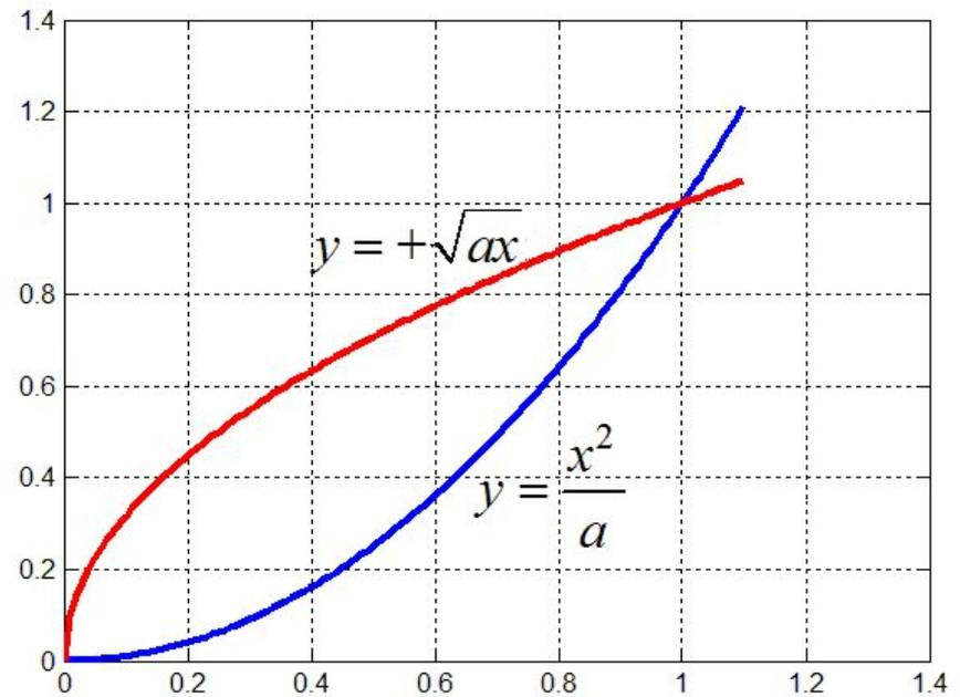
$$S = \int_0^a \left| \sqrt{ax} - \frac{x^2}{a} \right| dx = \int_0^a \left( \sqrt{ax} - \frac{x^2}{a} \right) dx = \sqrt{a} \frac{2}{3} x^{3/2} \Big|_0^a - \frac{x^3}{3a} \Big|_0^a =$$
