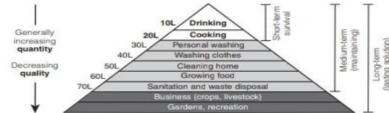
Figure 9.1. Hierarchy of water requirements (after Maslow's hierarchy of needs)
