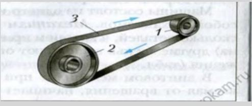
A 2D diagram of a belt drive. It shows two pulleys of different sizes (labeled 1 and 2) connected by a belt (labeled 3). Blue arrows indicate the rotation of the pulleys and the direction of the belt. |
