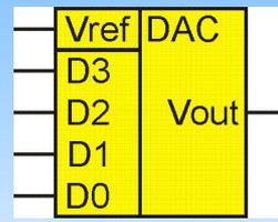
$$V_{out} \sim V_{ref} \times (code)$$
