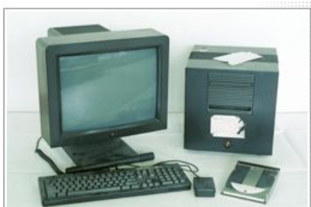
The historic NeXT computer used by Tim Berners-Lee in 1990, on display in the Microcosm exhibition at CERN. It was the first web server, hypermedia browser and web editor.
