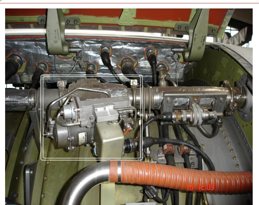
The inlet cowl anti-ice valve is an electrically controlled and pneumatically operated butterfly valve. It is spring loaded to the closed position.
