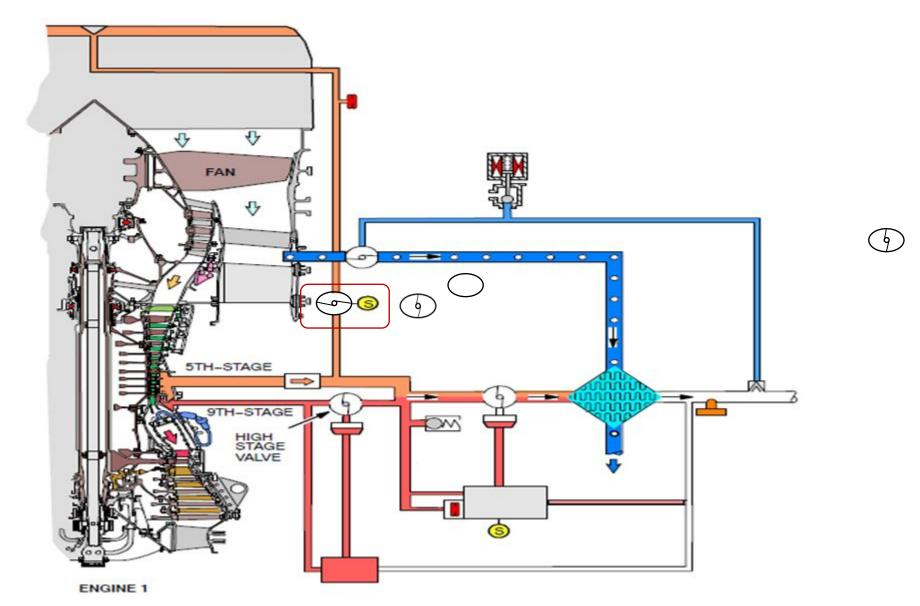
When the engine is runing, air comes and waits for selenoid activation to open the valve.
