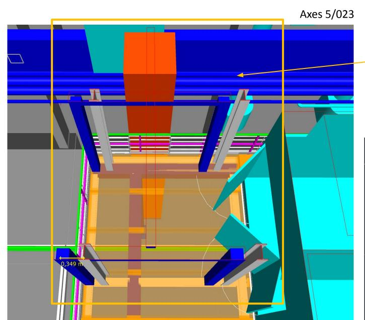
Move monorail columns 350mm left according to last gen. Layout (04/05) Otherwise ASU doors won't open correctly
