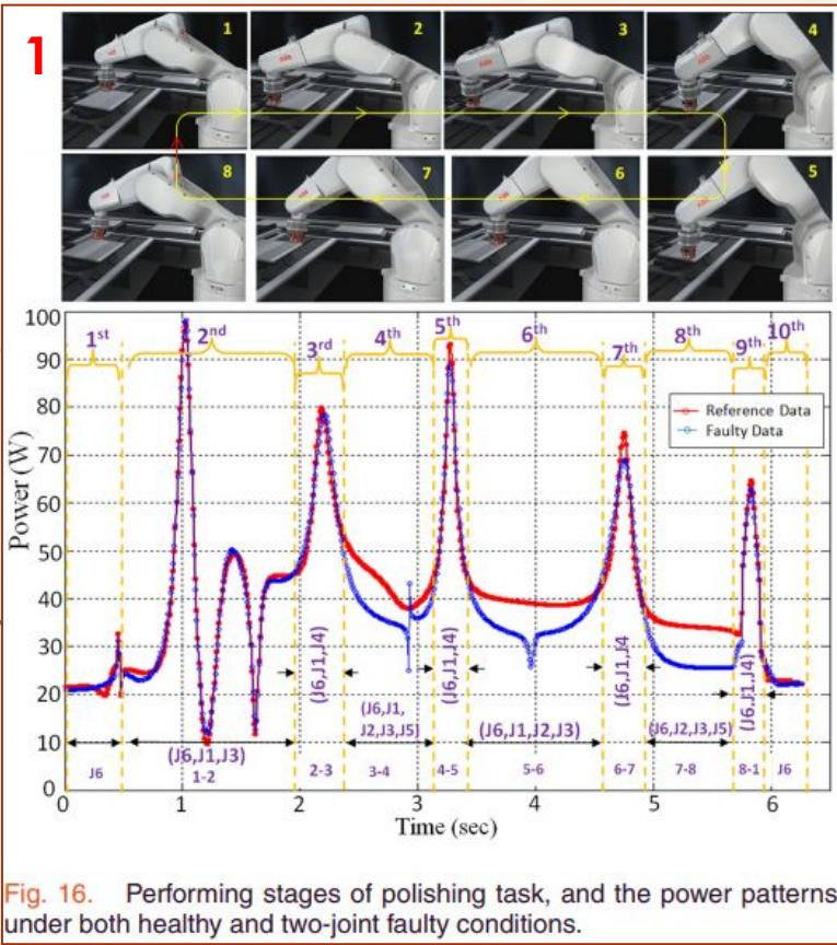
1 Fault Detection and Diagnosis of Industrial Robot Based on Power Consumption Modeling (TrInE20; Малайзия)
