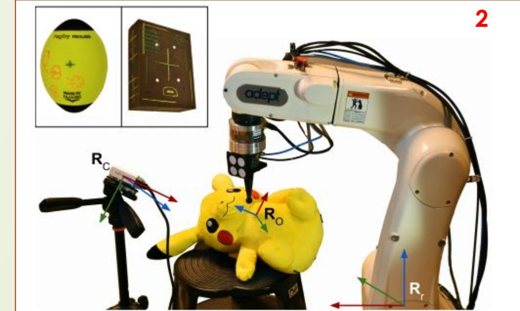
Fig. 4. Experimental setup showing the robot ( $R_r$ ) deforming a plush toy ( $R_o$ ) while the data is captured from an Intel RealSense D435 RGB-D Camera ( $R_c$ ). The other objects that have been experimented upon are shown in the inset above.
