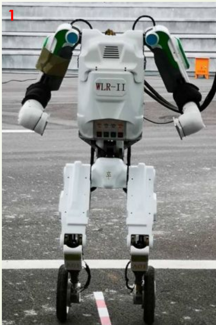
1 WLR-II, a Hose-less Hydraulic Wheel-legged Robot (IROS19; Hardin IoT)
