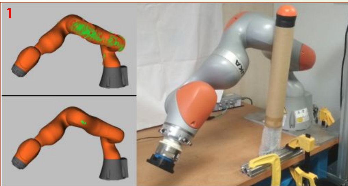
Fig. 7. Results in the real-world environment. Top-left: initial steps of the estimation before moving. Bottom-left: result of the estimation. Right: collision state (the robot's third link is colliding with a cylindrical obstacle).
