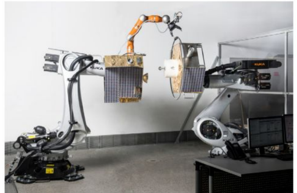
Fig. 1. The On-Orbit Servicing Simulator at DLR RMC: detail of the micro-macro space robot simulator.
