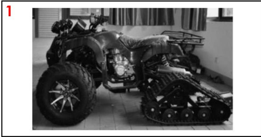
Figure 1. Structure of a coordinated variable wheel-track walking mechanism.
