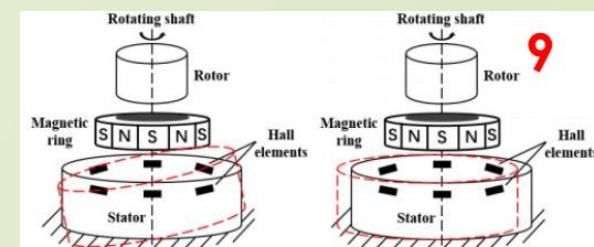
Figure 1. Tilt and eccentric error in manufacturing and installation.
