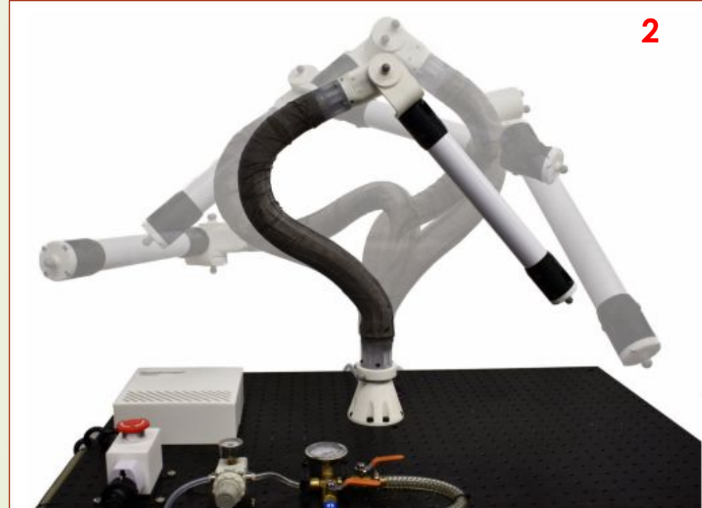
Fig. 1. The developed two-degree-of-freedom (DOF) malleable robot arm, showing various topology configurations it can achieve. A PUMA-like configuration is shown in foreground.
