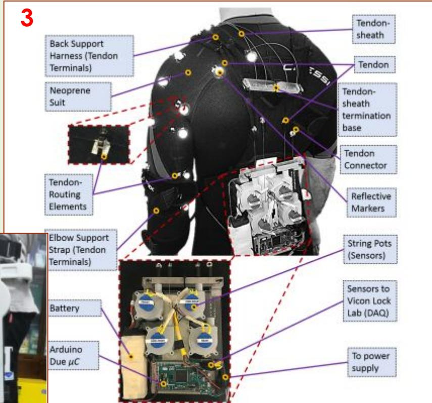
Overview of the sensing framework prototype for the shoulder exosuit description of the electro-mechanical and mechanical elements.
