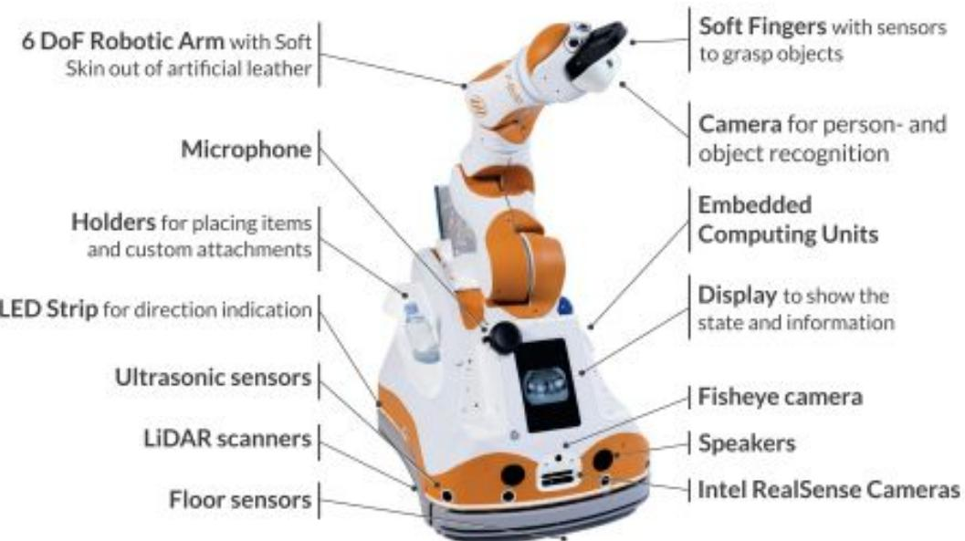
Fig. 1. Overview of Lio: sensor and hardware setup.
