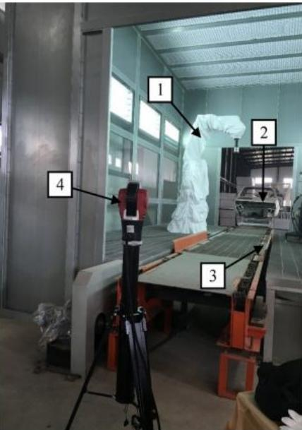
Fig. 13. The hybrid spray-painting robot is inspected by RQIC (1) Hybrid spray-painting robot. (2) Car shell. (3) Conveyor. (4) Laser tracker.
