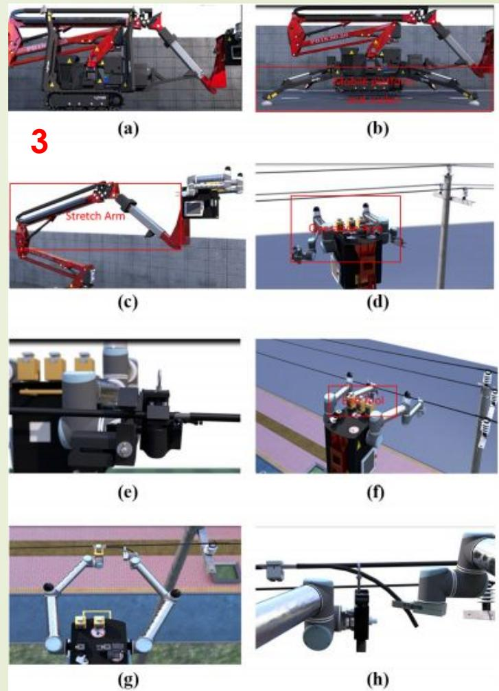
Notes: (a) Robot initial posture; (b) insulation arm starts rising; (c) insulation arm approach to working space; (d) both arms approach the working space; (e) stripping operation; (f) start working with both arms; (g) wire connection operation; (h) wire cutting operation
