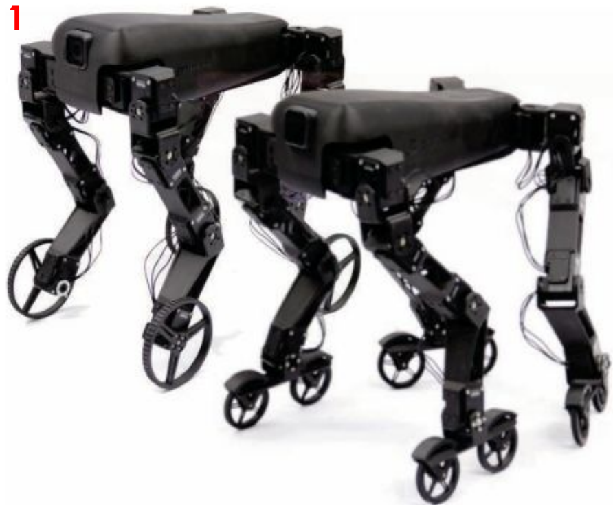
Fig. 1. AgileBot and SkaterBot, two robots created with the help of our interactive design system.
