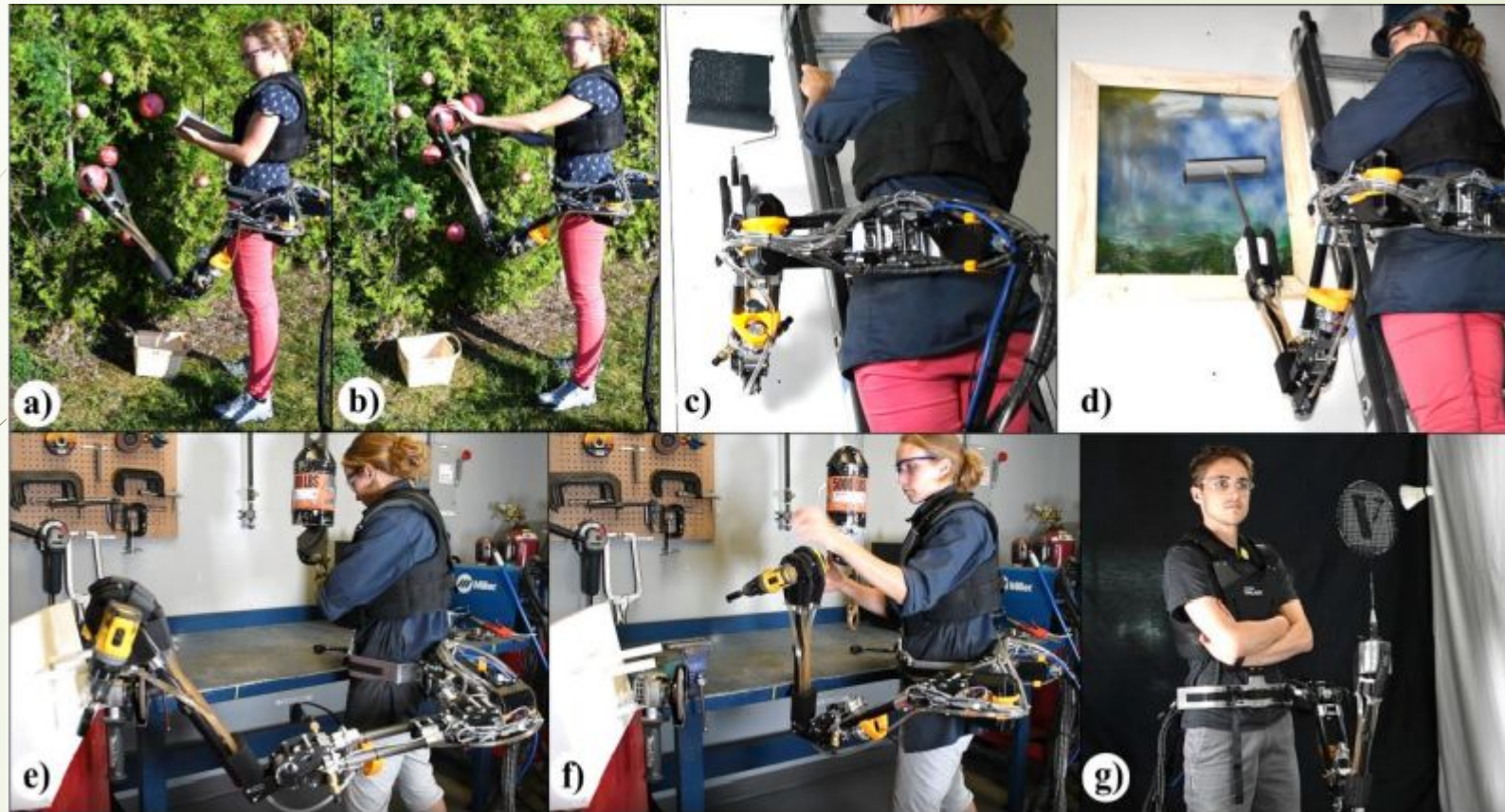
Figure 14. Variety of teleoperation applications with a SRL. a,b) vegetables picking, c) painting on a wall, d) washing a window, e,f) giving tools to a worker and g) playing badminton.
