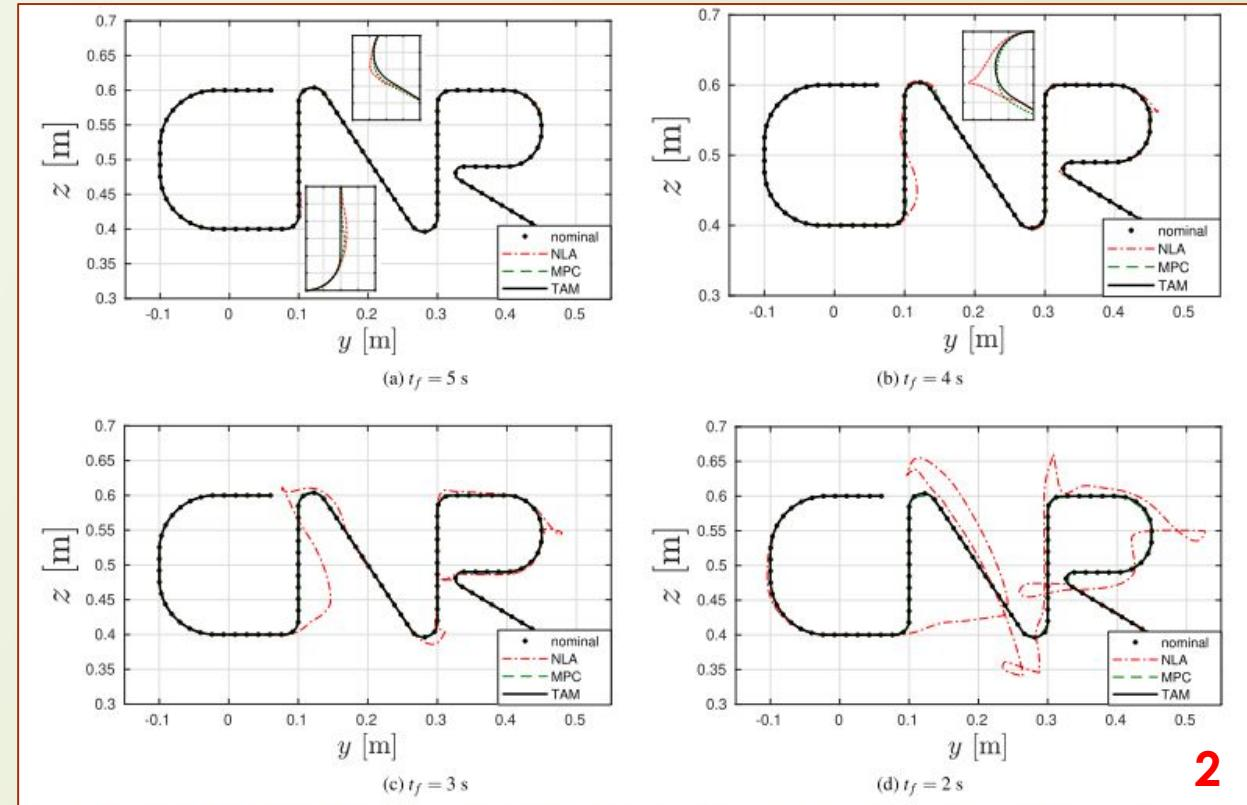
Fig. 4. Simulation results. Path performed by the different methods: nominal path (black dots); TAM (solid black lines); NLA (dotted red lines); MPC (dashed green lines). (For interpretation of the references to color in this figure legend, the reader is referred to the web version of this article.)
