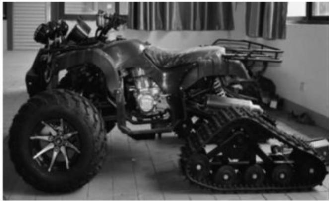
**Figure 1.** Structure of a coordinated variable wheel-track walking mechanism.
