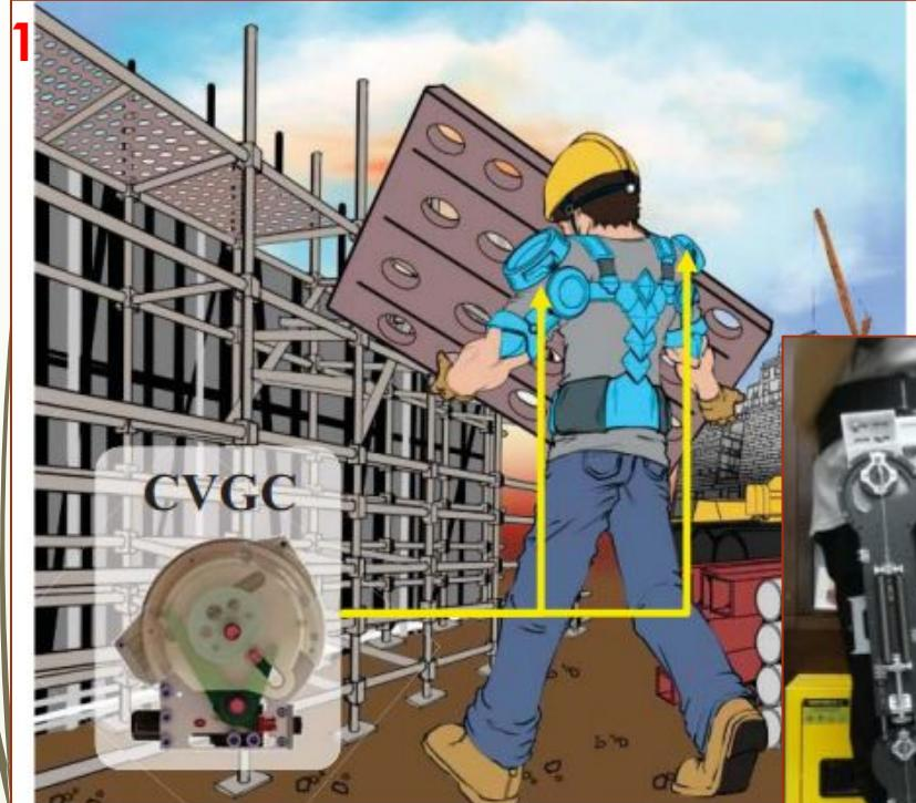
Fig. 8. Long-term application of the CVGC to passive-type wearable robots
