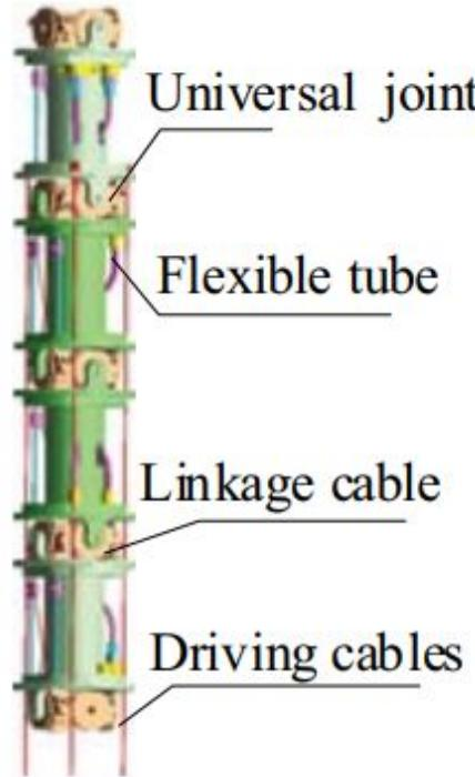
Fig. 2. The Preliminary Design of CRSM[9]
