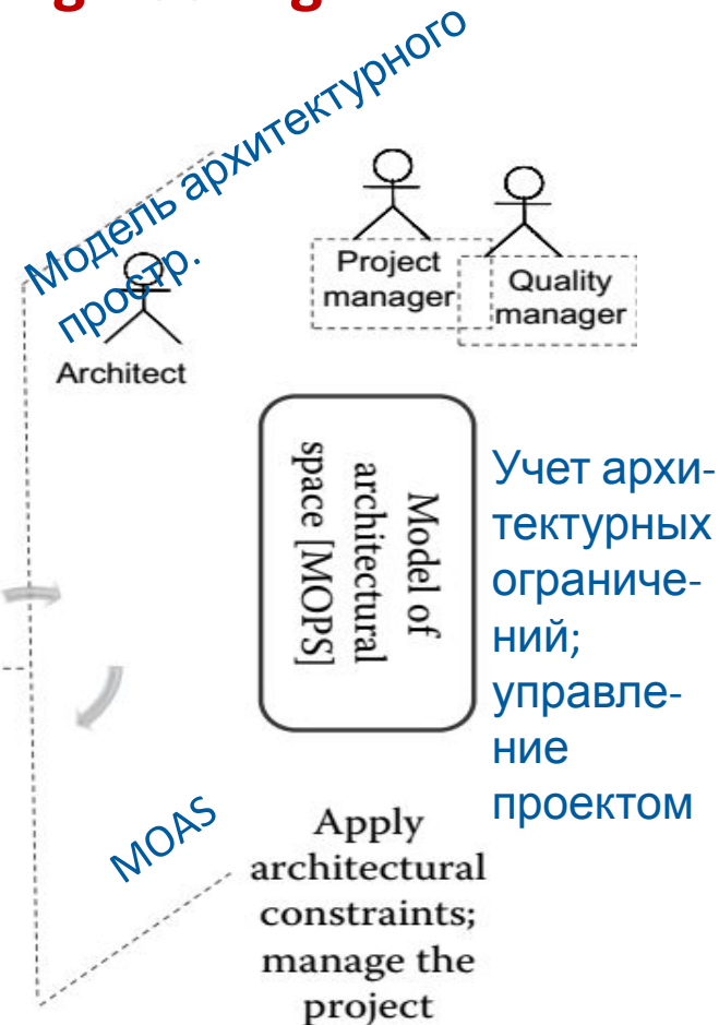
Figure 3.3 Software engineering uses three main modeling spaces and corresponding roles: model of problem space (in identifying the requirements and analyzing them), model of solution space (in creating the solution design), and model of architectural space (in applying constraints).
