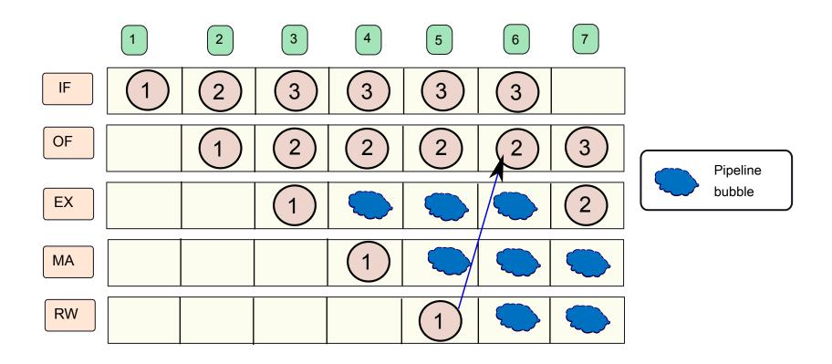
An interlock inserts a *nop* instruction (bubble) in the pipeline
