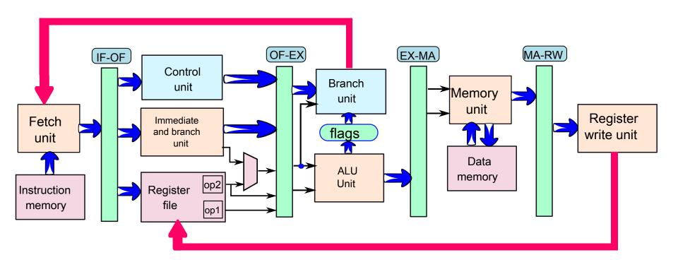
Note the positions of the pipeline latches.
