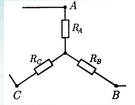
$$R_A = \frac{R_{AB} \cdot R_{CA}}{R_{AB} + R_{BC} + R_{CA}}$$
