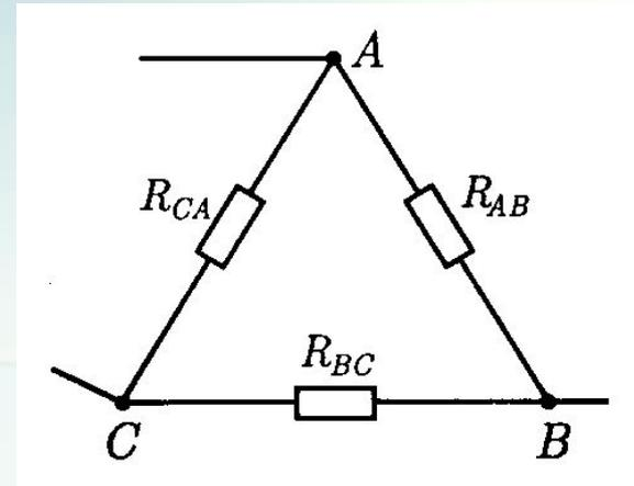
$$R_{AB} = R_A + R_B + \frac{R_A \cdot R_B}{R_C}$$
