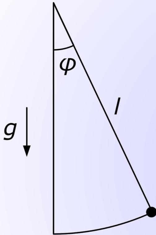
$$l \frac{d^2 \varphi}{dt^2} + g \sin \varphi + \mu \frac{d\varphi}{dt} = 0$$
