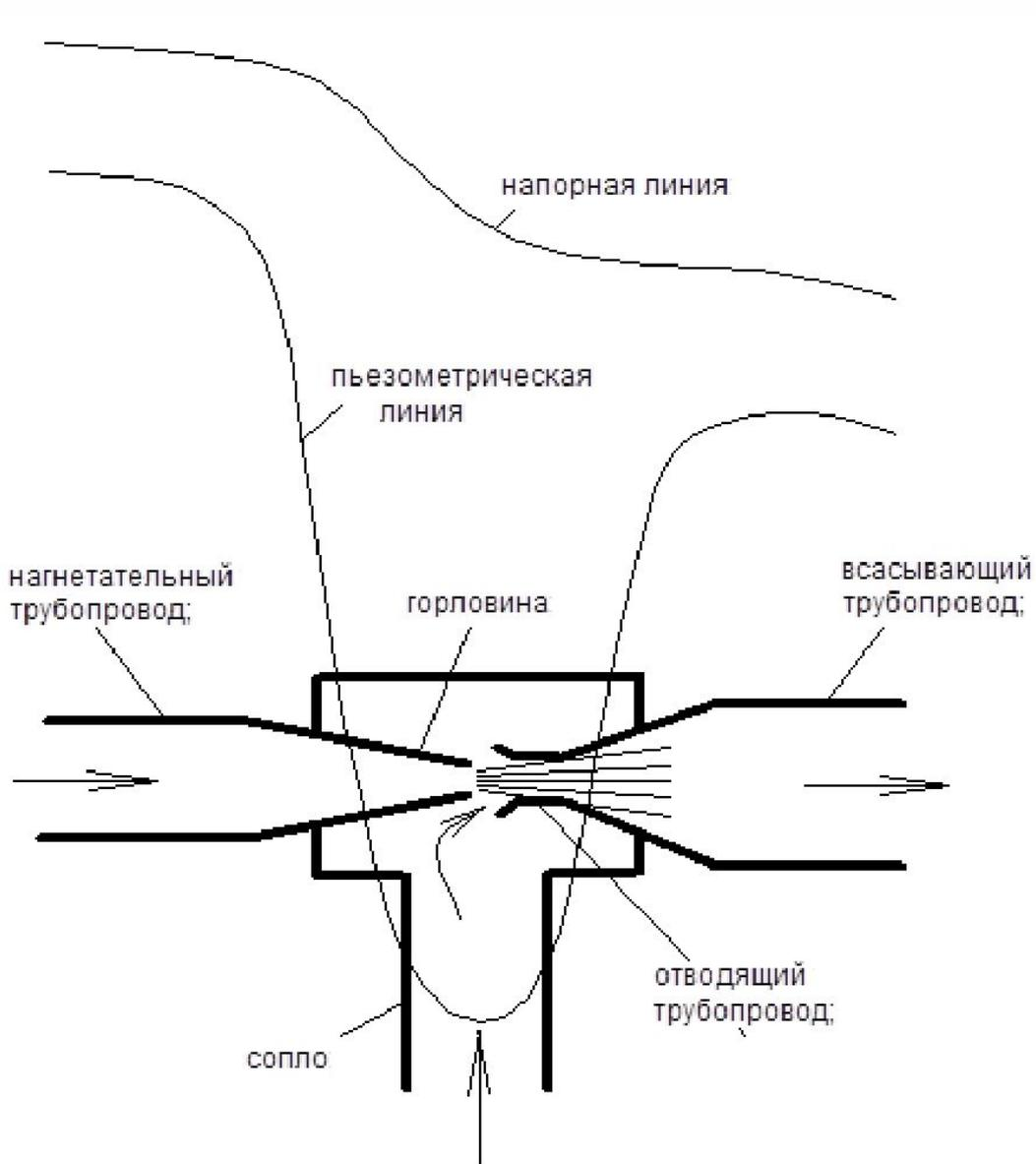
$$z_1 + \frac{p_1}{\rho g} + \frac{V_1^2}{2g} = z_2 + \frac{p_2}{\rho g} + \frac{V_2^2}{2g}$$
