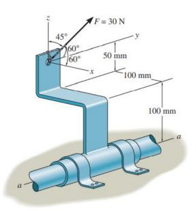
Replace the two forces and a couple acting on the bent rod ABC with an equivalent force-couple system acting at C.
