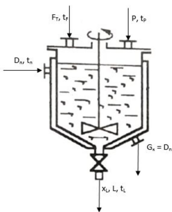
$$\Delta t_P = t_L - t_H \rightarrow t_L = \Delta t_P + t_H = 55 + 5 = 60^\circ\text{C}$$
