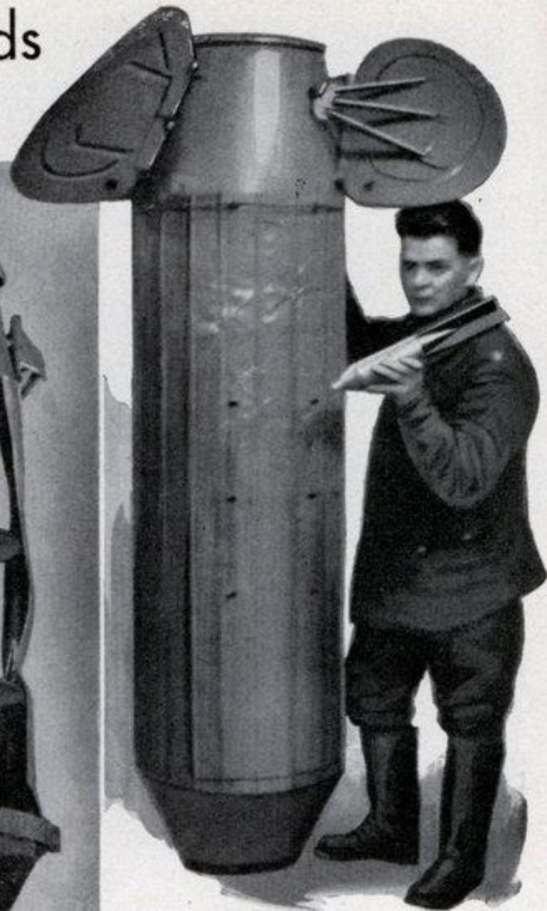
This huge case opens as it falls, throwing out the small bombs seen at the left
