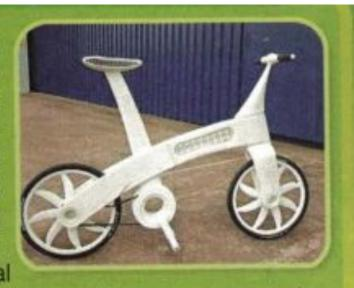
bicycle made of nylon called the Airbike. It's as strong as steel but much lighter. It comes out as a complete bike with no assembly required. The possibilities for this new technology are endless. Medical researchers hope that with a special cartridge of human cells and bio-friendly gel, it can be used to print out skin grafts for burn victims. They have already managed to demonstrate the potential medical uses by printing out a copy of a human ear in 30 minutes.
