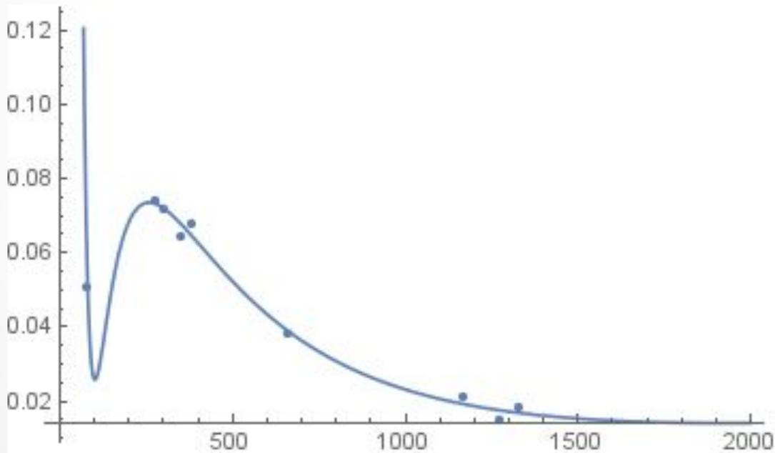
New approach for calibration the efficiency of HPGe detectors
