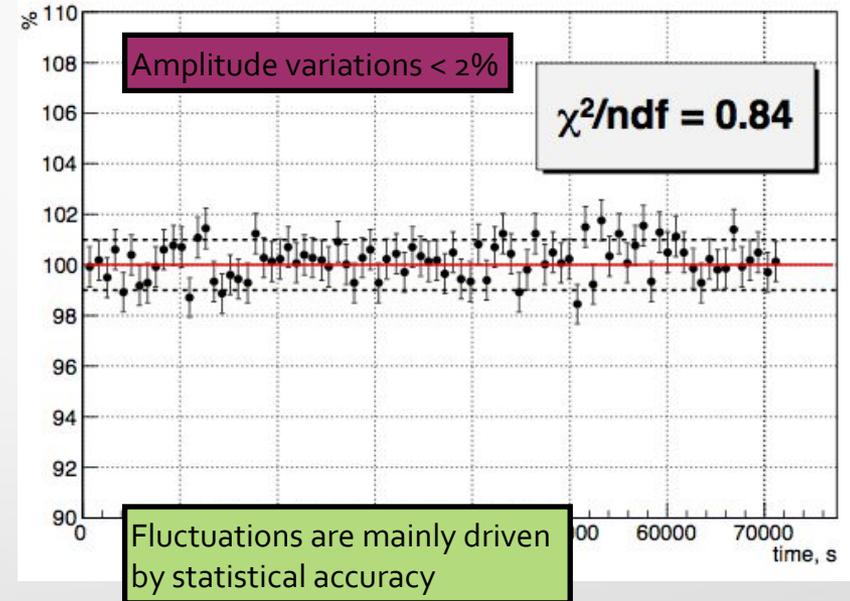
LED source stability measured by 20" Hamamatsu 12860 HQE PMT in a single point
