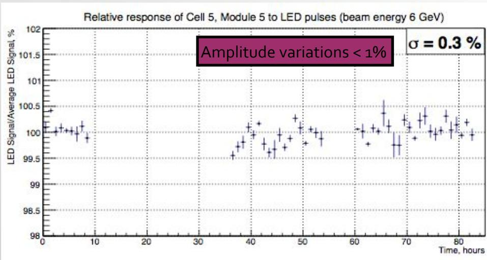
LED source stability measured by ECALo prototype for the COMPASS experiment (Has precise photosensor temperature stabilization < 10 mdeg) in june-july 2015 @ T10 (CERN).
