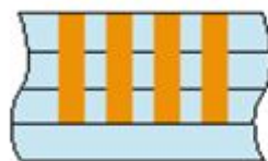
Blind thermal via for electrical isolation
