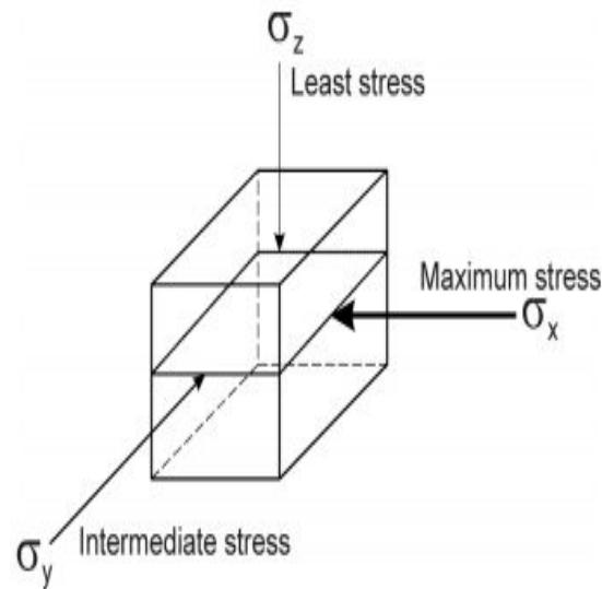
Figure 3-6a Horizontal fracture occurs when the least principal stress is vertical  $\sigma_z > \sigma_x > \sigma_y$  where the maximum stress is horizontal, a horizontal fracture will occur.
