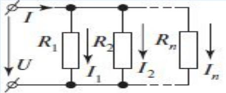
$I = I_1 + I_2 + \dots + I_n,$ <p>где <math>I_1 = \frac{U_1}{R_1} = U_1 G_1,</math></p> $I_n = \frac{U_n}{R_n} = U_n G_n$ |
