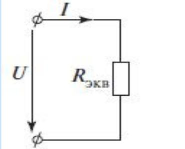
$I = \frac{U}{R_{\text{ЭКВ}}} = U G_{\text{ЭКВ}}$ |                         |
