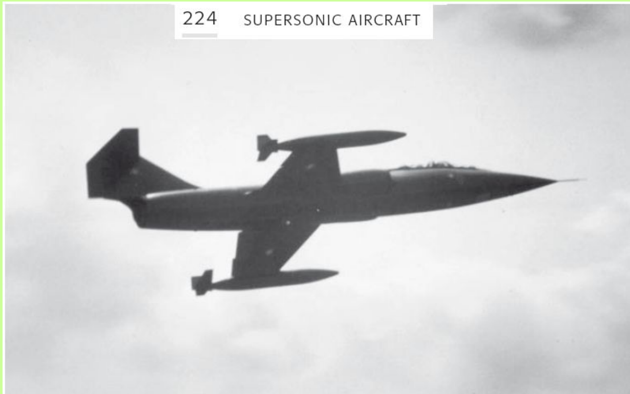
Fig. 8.8 Unswept wing for supersonic flight
